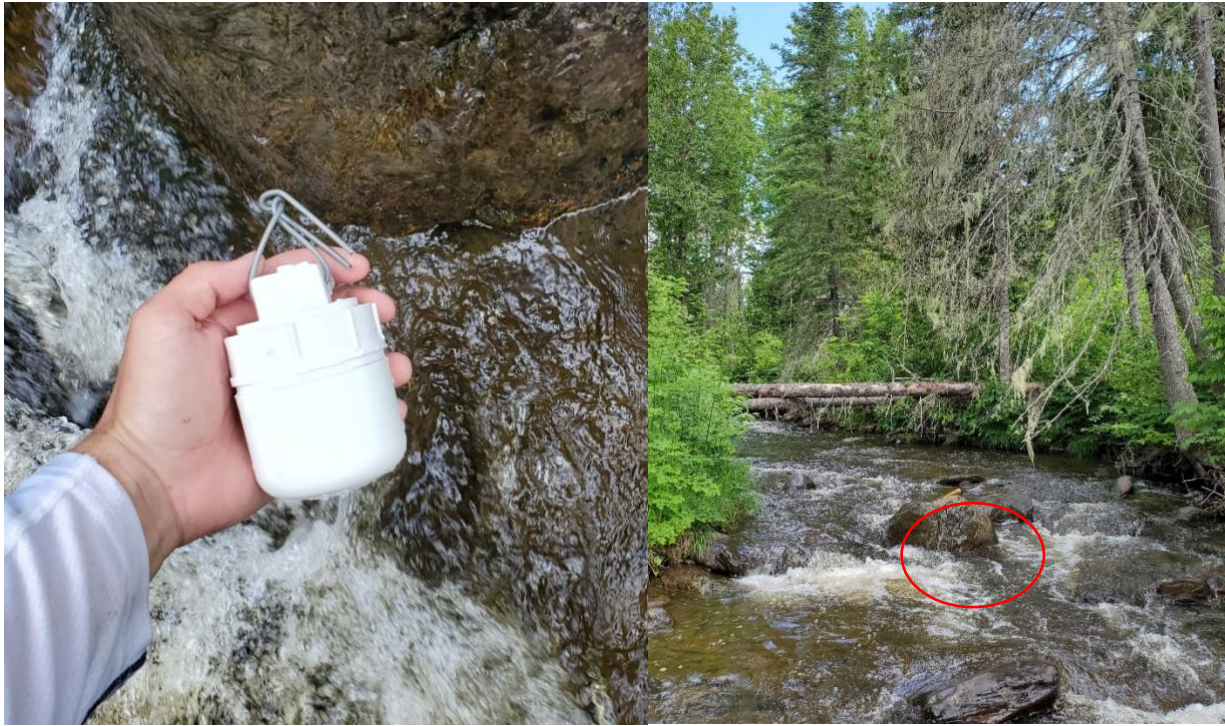
Figure 1: Temperature logger encased in PVC housing before deployment (left), and an example of a monitoring site behind a large rock in the middle of the channel (right).
