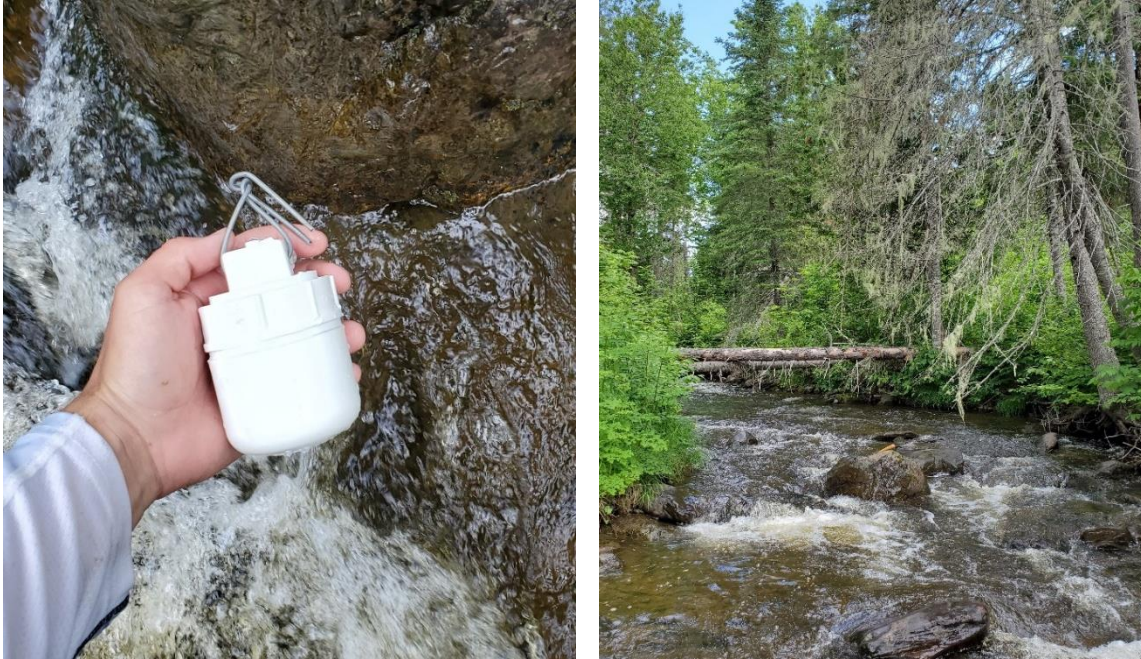
Figure 1: Temperature logger encased in PVC housing before deployment (left), and an example of a monitoring site behind a large rock in the middle of the channel (right).
